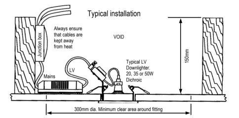
Transformer ratings Primary Voltage (Mains in) 240Volts 50Hz AC Primary running current 0.46 Amps Low Voltage (Secondary) 11.6 Volts AC 35-105 VA Low Voltage (VA) (Sec) Max. Sec Amps 8.8 Amps Isolation Class Class III SELV IP20 IP Rating Thermal 115°C Cut-off, resettable. Dimmable Yes
