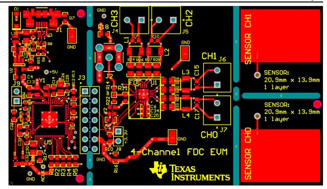
Figure 66. Layout Top Layer – Signals and Components
