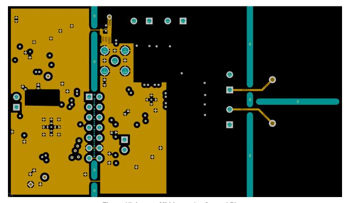
Figure 67. Layout Mid-Layer 1 - Ground Plane
