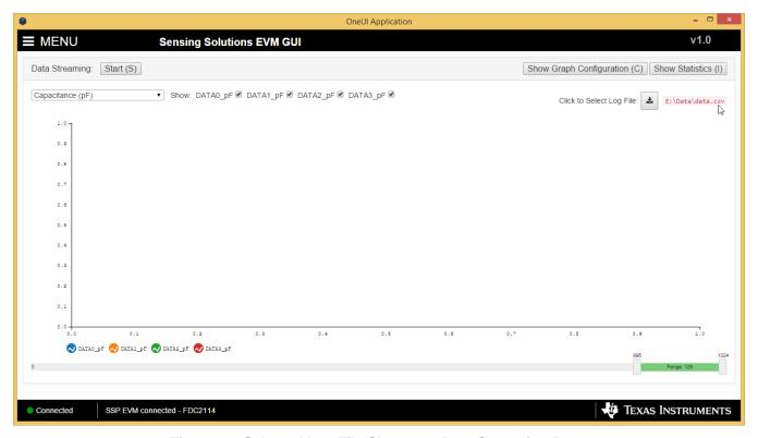
Figure 46. Selected Log File Shown on Data Streaming Page
