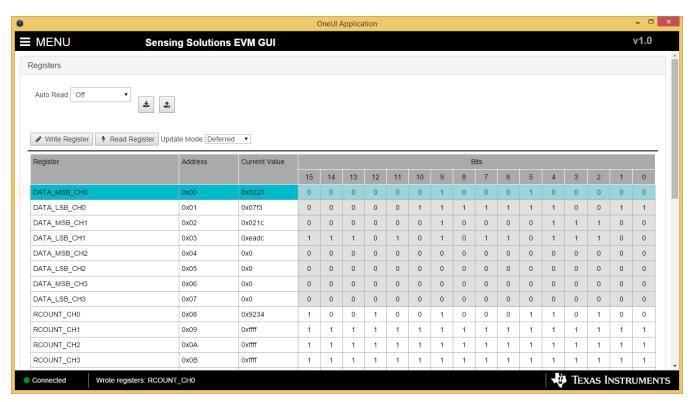
Figure 22. Selecting a Register on Register Page
