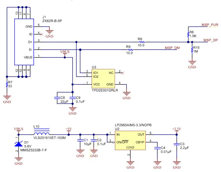
Figure 63. USB Connection and Power Circuit
