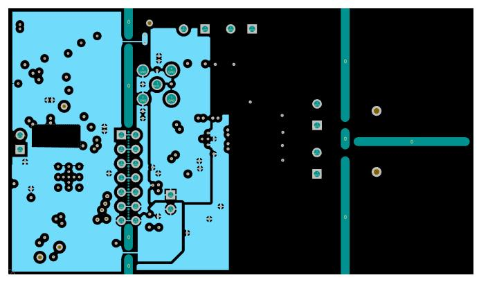
Figure 68. Mid-Layer 2 – Signals and Power Plane
