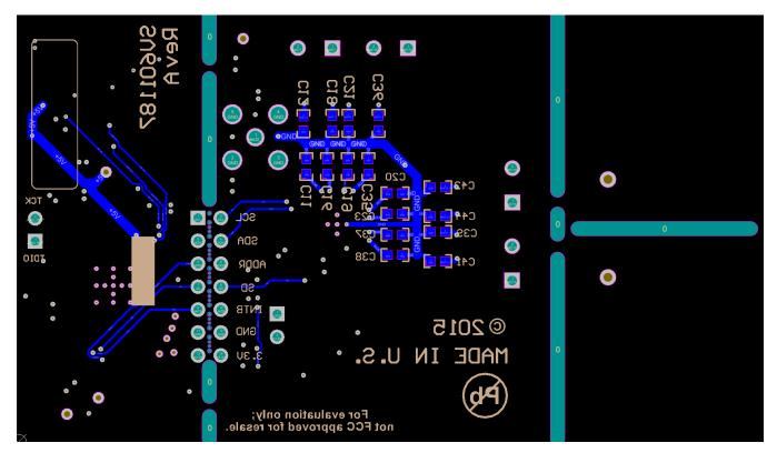
Figure 69. Layout Bottom Layer - Signals Plane
