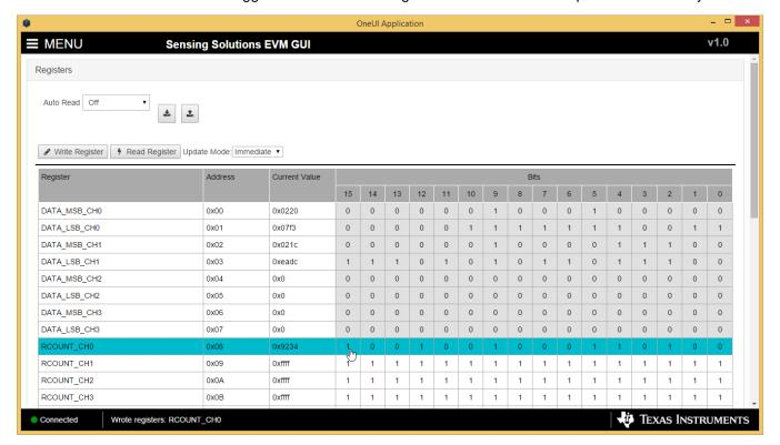
Figure 21. Toggling Register Bit Value on Register Page
