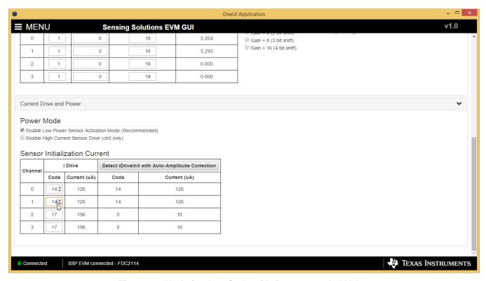
Figure 40. Updating I<sub>drive</sub> Code with Recommended Value
