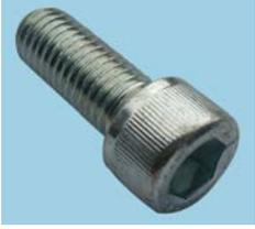
Din 912 Grade A4 ("acid proof") Stainless Steel precision manufactured fastener. Cap head with hexagon drive. Better corrosive resistance to aggressive media such as chlorides.
