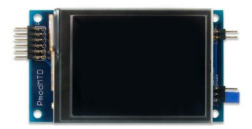
The Digilent Pmod MTDS (Revision A) is a gorgeous 2.8" touchscreen display with a powerful on-board microcontroller that performs graphics processing tasks. The display is a capacitive touchscreen with QVGA resolution (320×240) and 2 finger multi-touch support.
