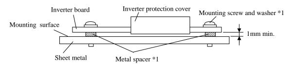
\*1: The conductive material (mounting screw, washer, metal spacer and so on) is allowed to mount within the limits of 3.5mm radius from the center of mounting hole.
