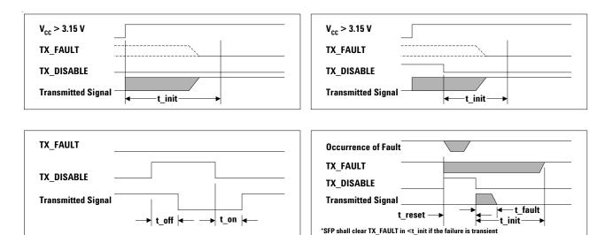
Figure 5 - Transceiver timing diagrams
