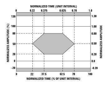
Figure 6 - Gigabit Ethernet Transmitter eye mask diagram
